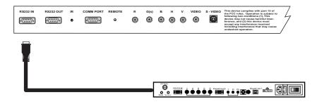
The projector has a RS232 port that allows it to communicate with the VHD Controller.
